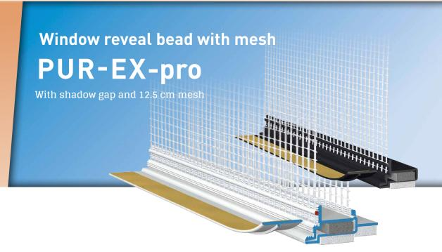
The **APU window reveal bead with mesh PUR-EX-pro** is used in compound heat insulation systems as specified in the latest APU selection criteria. Within the reveal the profile is stuck flush to the structural element there and thus forms a clean and reliable termination of the plaster with shadow gap.
